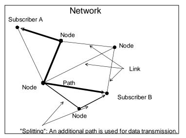
The nodes in between subscriber A and Subscriber B must ensure a "switching service", so that the message sent by A reaches B. This is comparable to relaying calls in a public telephone network.
