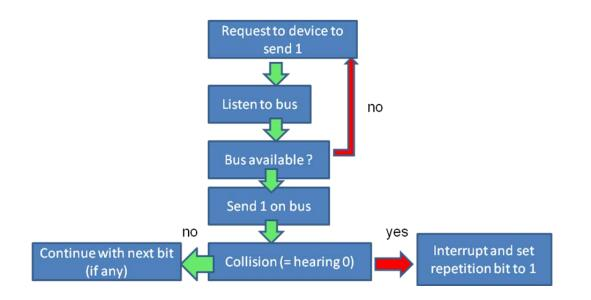
Telegrams of the first and second priorities as well as repetition telegrams can be transmitted immediately when the Layer 1 indicates that the bus is available, whereas messages of the lower priorities are delayed by the time  $t_1$  (= 3 bit pulses).
