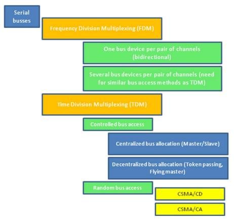
Figure 2: Classification of Serial buses
