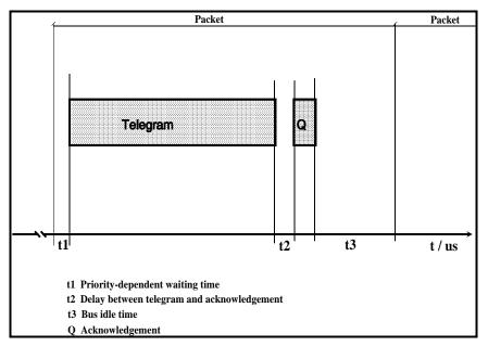
The total time  $t_{tot}$  required for the transmission of the telegram and the acknowledgement and the observance of the bus idle time is calculated as follows:
