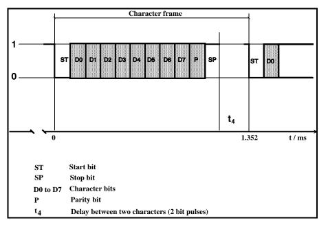
The protocol foresees a transmission break  $t_2$  of at least one character width after the sending of the entire telegram. The next character width is reserved for the reception of acknowledgement, which must be sent by the addressed bus devices of the link or of the line coupler / backbone coupler / line repeater.
